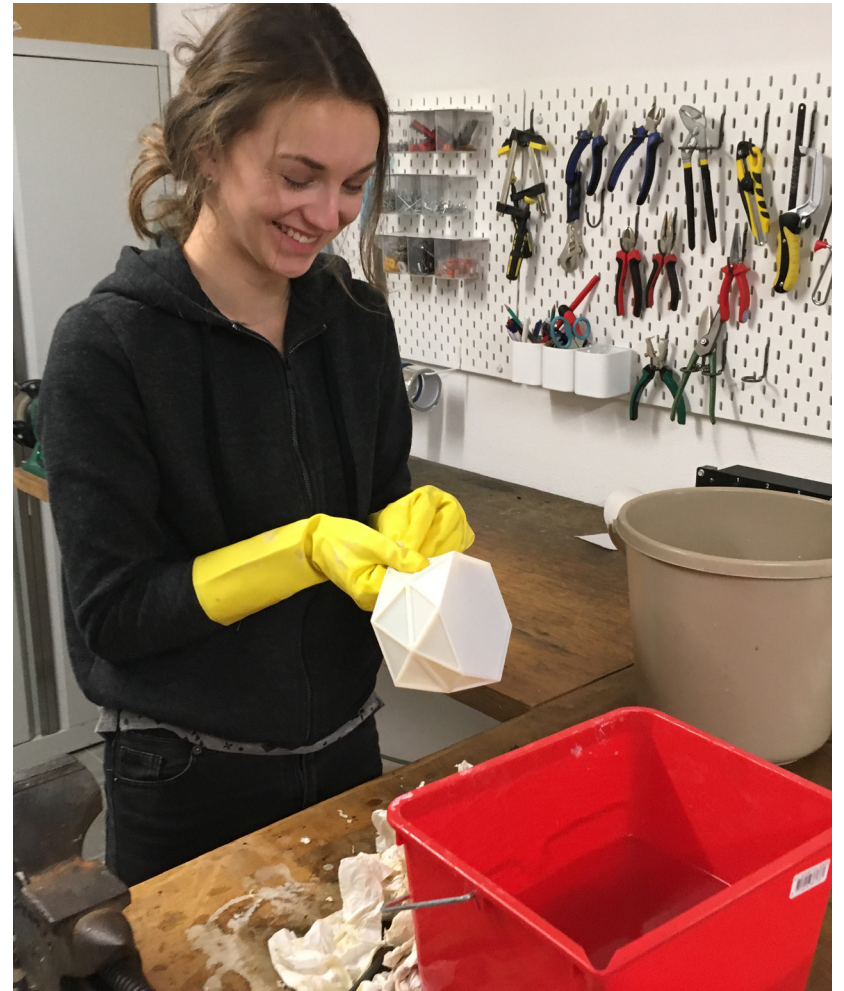
figure 6.16: using caustic soda to remove Objet support
